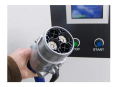
Fast charging differs from slow charging also in that it uses DC (Direct Current) instead of AC (Alternating Current).
