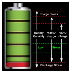
The life of a battery is reduced when at extreme high or low levels of charge<sup>37</sup>. To avoid cars reaching either end, not all of the battery capacity is made available.
