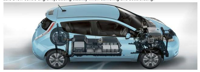
Battery size is measured in kilowatt-hours, or kWh. Lower priced electric cars have ~24 kWh batteries and the high-end Tesla Motors cars come close to 100 kWh. This affects range and cost.
